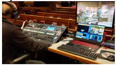
Preparing a Grace Livestream Worship - Bruce and Mary Stephens are at the computers showing the <u>VMix</u> <u>software</u> that takes the input from the <u>two PTZOptics</u> <u>Broadcast cameras</u> for producing the video data stream. The computer, cameras, and software were funded by the
